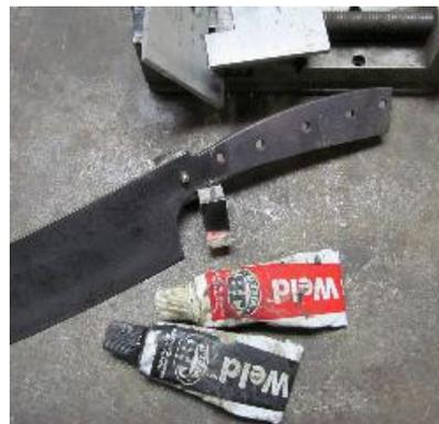
Go to the anvil and set the rivet. If all is well, the bolsters are now level with the shoulders of the tang, are parallel to one another and are locked down to the blade. Remove excess JB Weld with acetone, paper towels and the edge of a tongue depressor (or Popsicle stick). Don't forget to clean the alignment plates.
