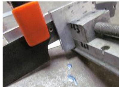
Position the correct block (here the right side one) with the polished face forward and the milled angle face to the blade and use a transfer punch to mark the location for the rivet hole.
