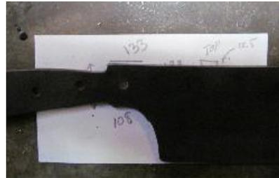
The difference divided by two determines the shim amount needed to compensate for the bevel and to keep the outer surfaces of the blocks parallel to each other and the center line of the blade. Here it is 12.5 thousands.
