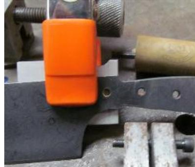
Transfer that position to the machinist vise and alignment plates. The alignment plates are better shown in an image to follow.
