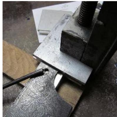
Once the positions are marked (indicated by the white arrows), it is off to the drill press to make 1/8" holes in the blocks. Since the marks are on the angles faces, the holes will be parallel to the outer faces (or as good as your drill press can do).
