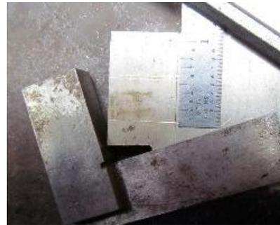
Mill the front & back surfaces of both blocks together to make the width of the blocks identical to one another.
