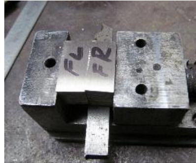
Measure the thickness of the blade at the spine and the belly (here 0.133" & 0.108" respectively). This is a measure of the taper of the bevel at the bolster point.
