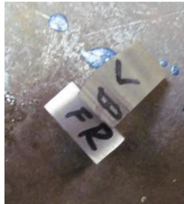
Then it is back to the mill to add the correct angle to the block's inner faces. We need 12.5 thousands & a business card is about 10. Shim the top face so that the mill will cut that face deeper than the bottom face.
