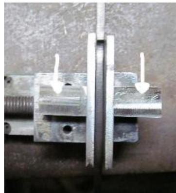
It is a good idea to chamfer the outer end of the hole to allow the rivet to spread and lock the blocks down when the rivet is hammered.
