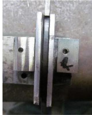
The front faces are given a final polish to remove any marks left by the drill press vise.
