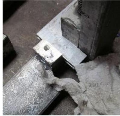
If needed, grind off any rivet that protrudes and clamp the blade in a decent vise as shown. Depending on air temperature, expect to wait until the next morning before moving onto the pommel & handle tasks.
