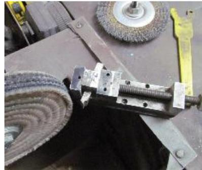
The alignment plates key over the vise on their lower horizontal surfaces and have machined parallel vertical edges. The blade tang will be sandwiched between the plates and will abut the rear surfaces of the bolster blocks.
